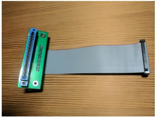
One example of a finished cable and adapter. The orientation of the connectors, and thus the orientation they "leave" the adapter is up to you and how you assemble the cable.
